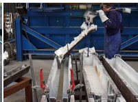
Figure 9 : Coulage anodes - Copenhague Danemark
